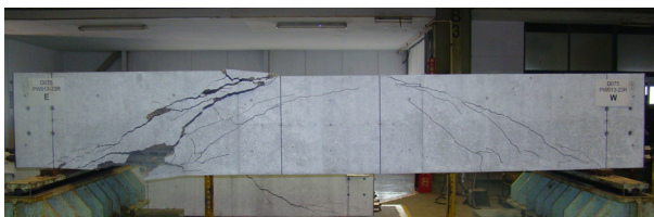
Photo 7 実験終了後のひびわれ状況 (D075PW013-23) Side View of Tested Specimen
