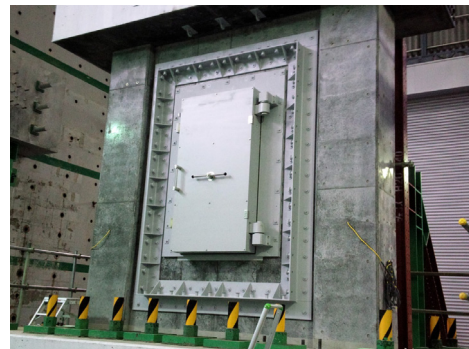
Photo 1 RC 造耐震壁に設置した水密扉 Watertight Door on RC Wall Specimen
