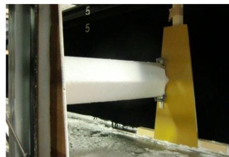
Photo 2 着雪状況例 (Case2(H=200mm)) Example of Snow Accretion to the Flat Plate (Case2)
