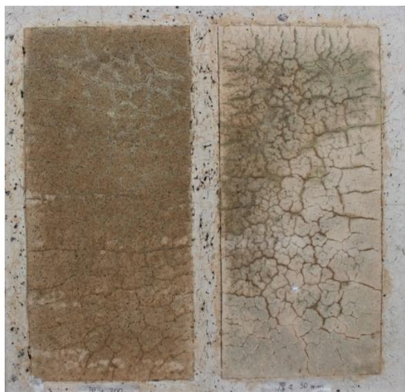
補修厚さ30mm 補修厚さ200mm
