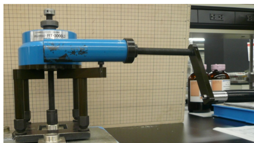
Photo 1 油圧式簡易引張試験器 Simplified Hydraulic Pulling Adhesion Test Machine
