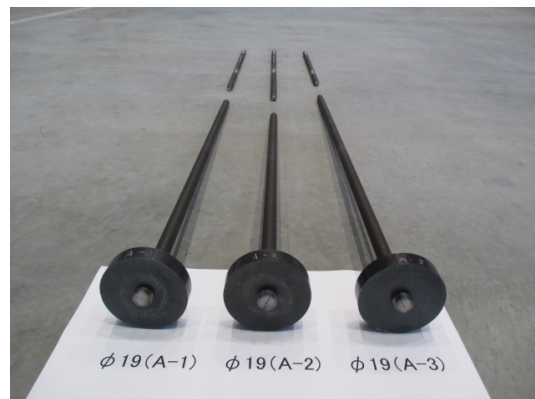
Photo 4 破断状況 ( \phi 19 ) State of the Nut-Bar after the Test-A ( \phi 19 )
