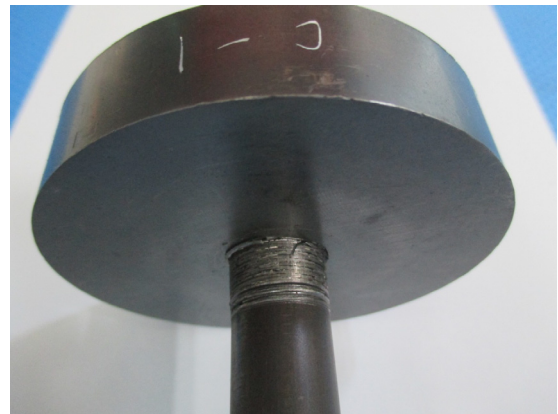
Photo 5 嵌合部のおねじ破壊状況 (φ19) The External Thread Failure at the Joint (φ19)
