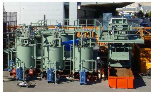
Photo 3 鉄粉洗浄の設備 Devises of Washing Remediation Using Iron Powder
