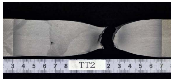
Photo 4 溶接継手引張試験結果例 Example of Weld Joint Tensile Test Results
