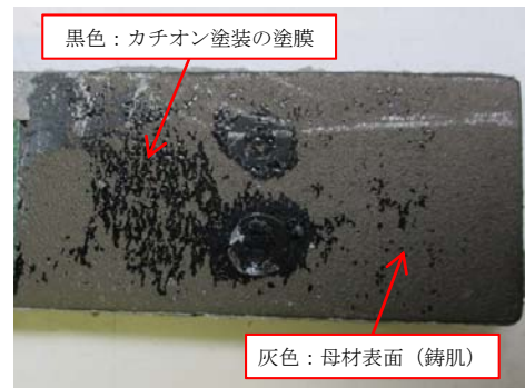
Photo 1 接着面破壊状況 Failure Pattern on Bonded Surface
