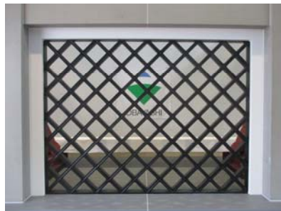
Photo 7 実大試験体 Mock-up of Casting Block Wall
