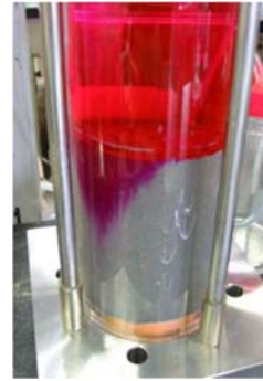
Photo 3 界面未対策時の透水試験の漏水状況 Permeability Test without Measures against Leakage
