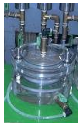
Photo 2 透水試験 Permeability Test using φ10cm Mold
