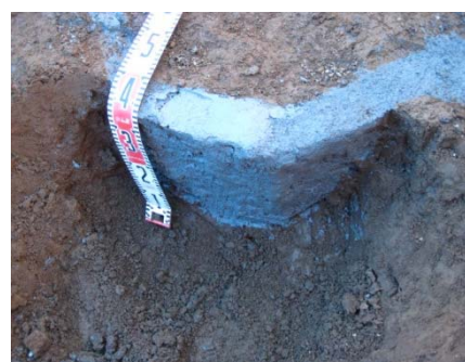
Photo 7 鋼矢板の引抜き後の注入断面 Cross Section of Discharge Material
