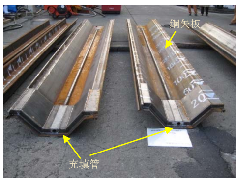
Photo 4 鋼矢板と充填管 Sheet Pile with Injection Pipe
