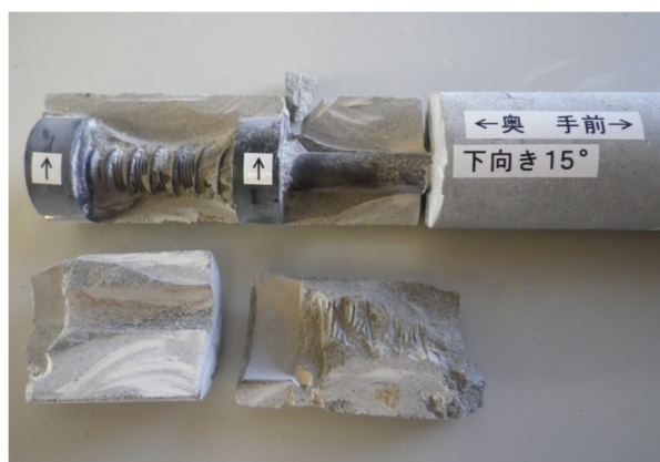
Photo 10 斜め下向き施工におけるモルタル充填状況 Filling Status in case of Downward Slope Grouting
