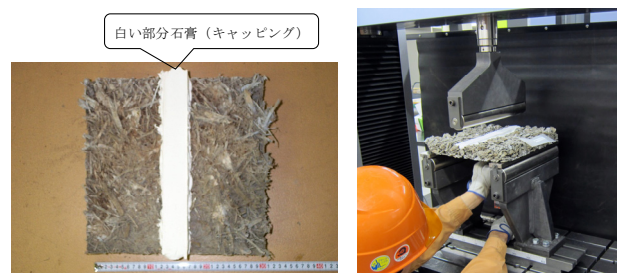
Photo 5 曲げ試験の供試体と試験状況 Test Piece and Situation of Bending Test
