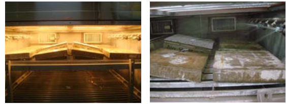
Photo 3 赤外線ランプ照射と散水の繰返し試験 IR-Irradiation and Water Showering Cycle Test
