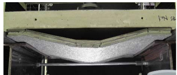
Photo 6 押抜き試験の状況 Appearance of Punching Load Test
