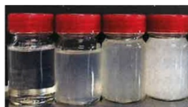
Photo 2 混合樹脂の相溶性試験結果 Results of the Mixed Resin Compatibility Test
