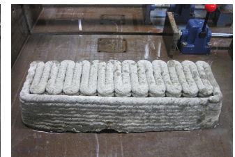
Photo 4 切出し前(垂直) Before Cutting(Vertical)
