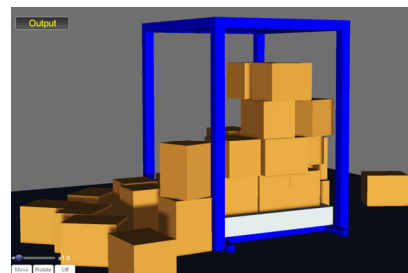
Fig. 7 積荷・什器類の地震時挙動シミュレーション Physics Simulation of Stacked Cargoes and Furniture due to Seismic Motion
