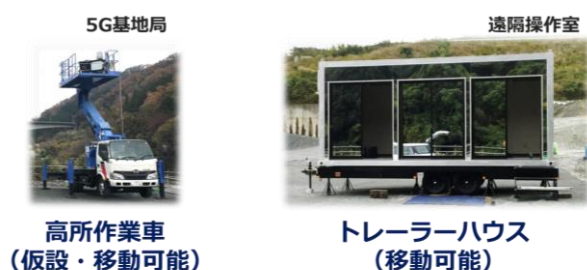
Fig. 2 5G基地局および遠隔操縦室 5G Base Station and Remote-Control Cabin
