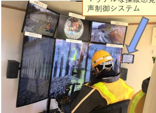
Fig. 10 音声制御(オペレータ1名で2種類の重機を操縦) Voice Control System (One operator controls two types of heavy equipment)
