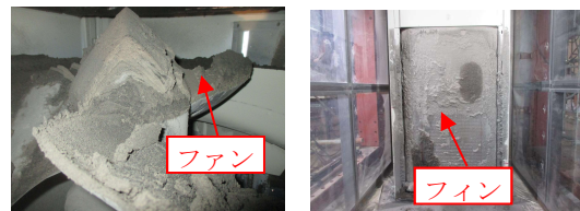
Photo 2 空調室外機に付着した火山灰(実験 3~4) Volcanic Ash Attached to Exterior Section of Air Conditioning (No.3~4)
