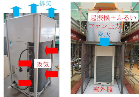
Photo 1 空調室外機と実験装置 Exterior Section of Air Conditioning and Experimental Equipment
