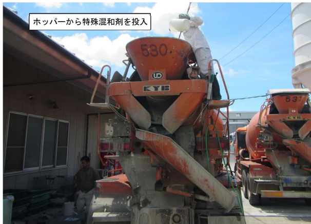
Photo 3 特殊混和剤の添加の状況 Situation of Special Chemical Admixture into Agitator Car
