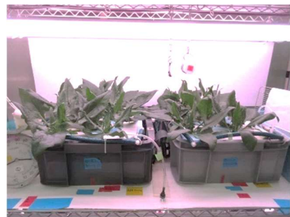
Photo 4 遠赤領域強化白色LEDによる育成 Cultivation Situation of the Spinach by Far-Red Light Reinforcement White LED
