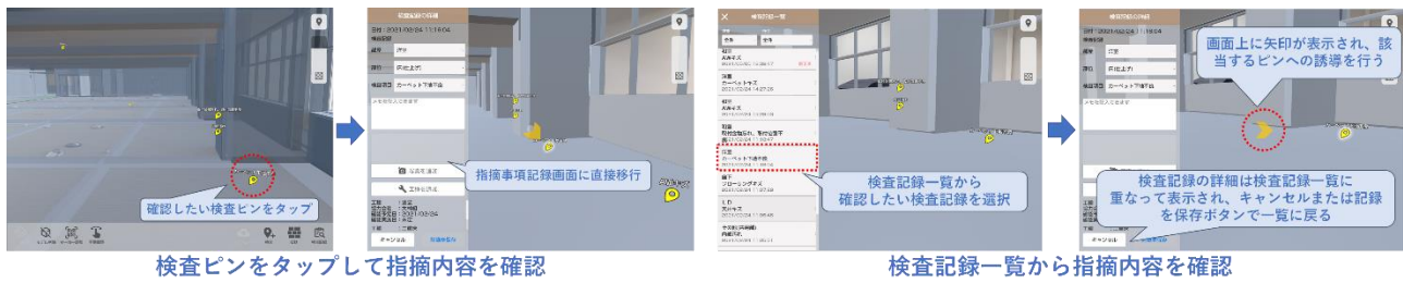
Fig. 10 指摘内容確認の操作性向上のための追加機能 Added Features for Improving Usability of Confirming Inspection Record
