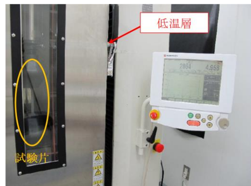
Photo 8 低温環境下の試験状況 Tensile Test in Low Temperature Environment
