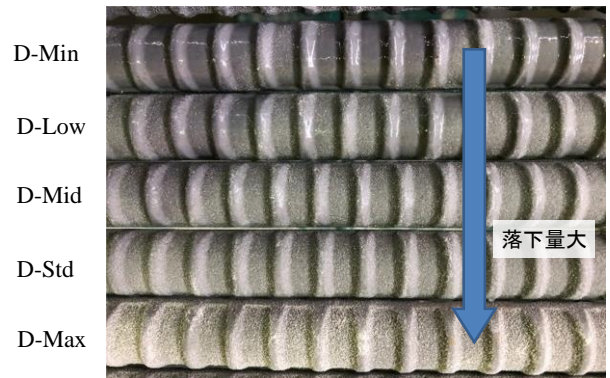
Photo 5 珪砂の付着状況 Silica Sand Adhesion Condition
