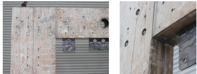
Photo 4 加熱実験後の状況 Surface of Beam-Column Joint after Fire Test
