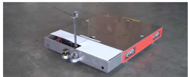
Photo 3 低床式AGV Autonomous Low-Fatbet AGV
