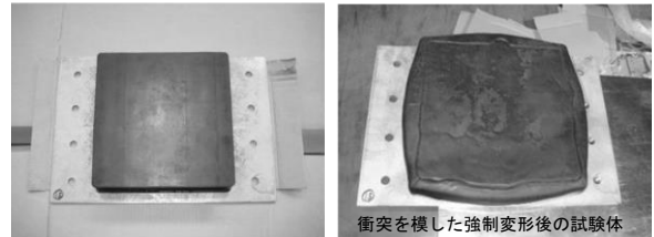
Photo 1 免震フェンダー (左：載荷前、右：載荷後) Menshin Fender (Before and after loading)
