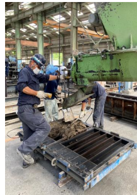
(1) 打込み Concrete Placing
