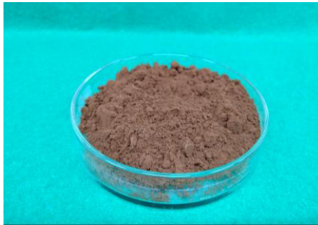
Photo 2 リグニン粉末の外観 Appearance of Lignin Powder
