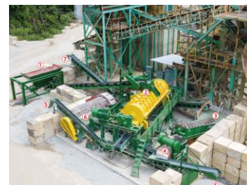
Fig. 2 再生骨材製造工場および製造フロー Recycled Aggregate Manufacturing Plant and Manufacturing Flow
