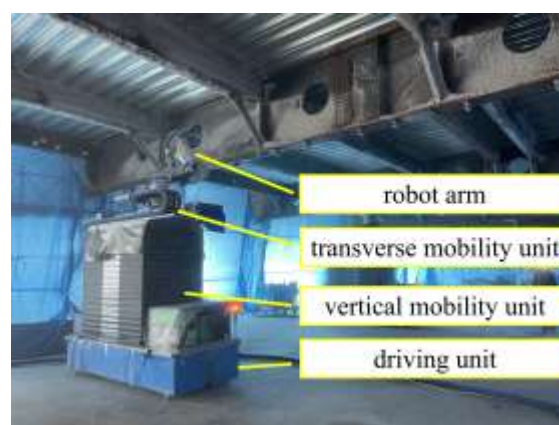
Fig. 1 Fireproof coating spraying robot
