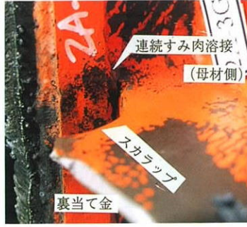
(2) 裏当て金の連続すみ肉溶接の重なり Continuous Fillet Weld Overlapped at Tack Welding of Backing Bars
