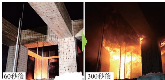
柱・梁が木あらわしの場合の火災の燃え広がり Fire Spreading of Wooden Buildings with Bare Beams and Columns
